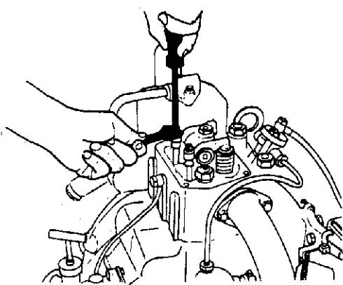
※ First obtain the proper bolt position for maintaining the required clearance with a screwdriver; then tighten the nut with a wrench.
