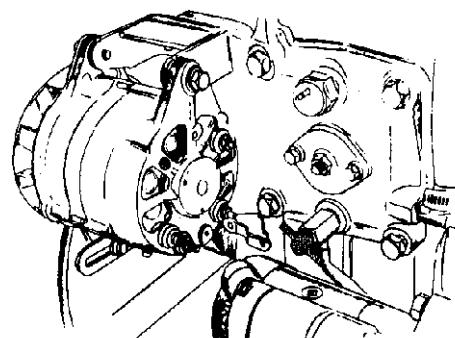
[5-3] Remove both inlet and outlet hoses from the cooling water pump, then turn the engine thru several times with the starting handle to discharge water from inside the cooling water pump. After following the above procedure, connect both hoses as before.
