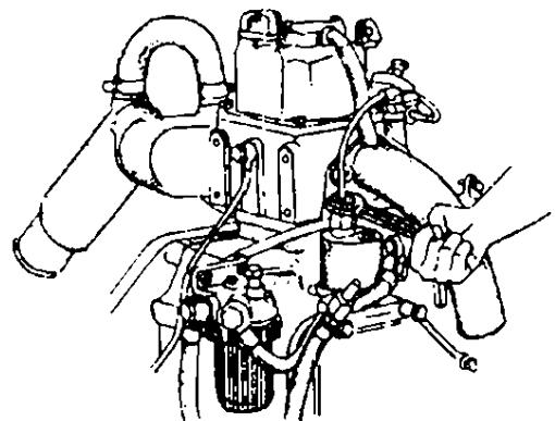
*By this procedure, air can be completely vented from the fuel line.*
